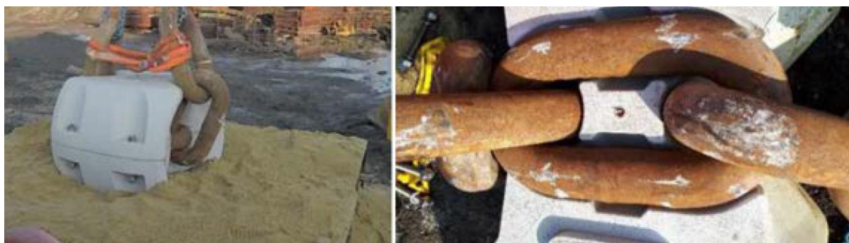
Figure 16 – WindFloat Atlantic clump weight testing from OTC 31744. It is noted the system was installed in 2019.
