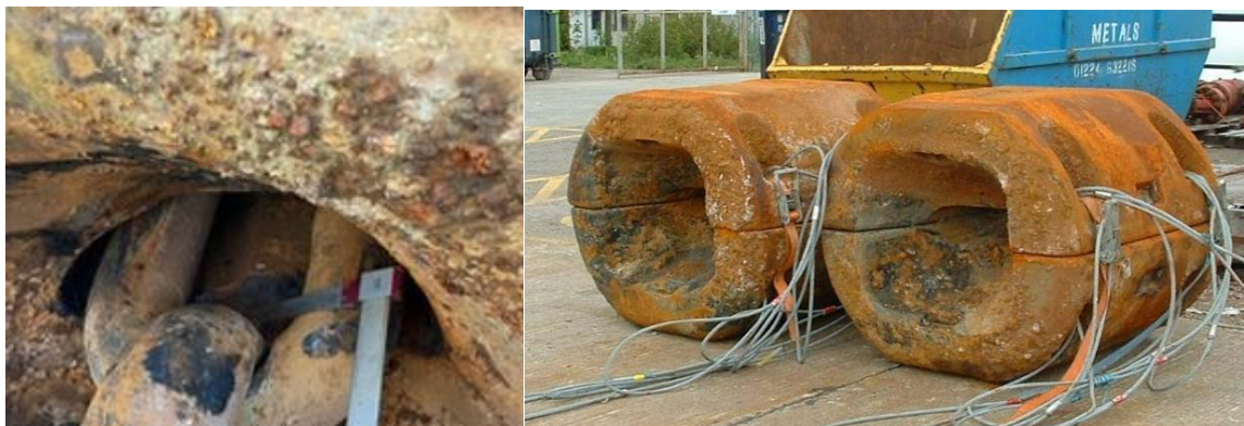
Figure 15 – High wear inside FPSO mooring clump weights and recovered clump weights from 2006 HSE RR444 report
