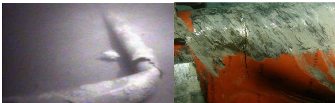
Figure 46 Kinked and cracked pipelines following Hurricane MODU run-over [25]
