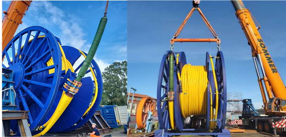
Figure 5 Dynamic cable pre-terminated for the Provence Grand Large FOW project [7]
