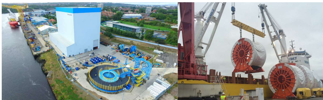
Figure 6 (left) Onshore cable load-out at TechnipFMC's Newcastle facility [8]; (right) Load-out of cable reels onto a cable lay vessel [9]
