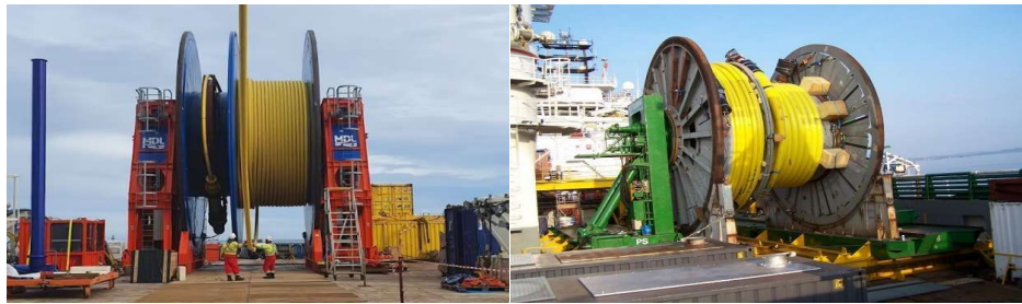
Figure 2 Two separate reel drive examples by (left) Maritime Developments Limited [24] and (right) Huisman [25]
